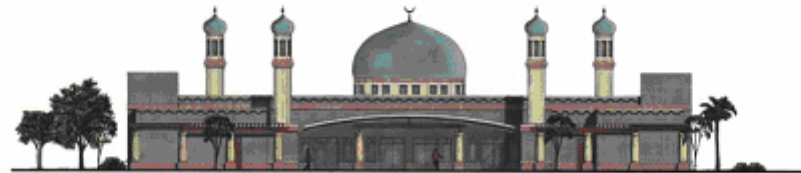
MOSQUE ELEVATION FROM COURTYARD SCALE: 1/8"=1'-0"
